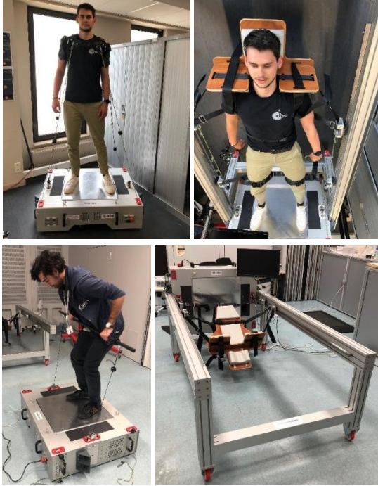
Figure 3. NEX4EX exercises modes (Top-left to bottom-right: Postural training, Plyometric training, Resistive exercise and MGSE ground test platform)
